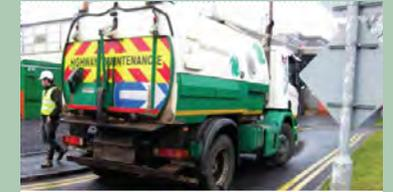
**03** Use a road sweeper with a recirculating water system
